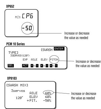
Once this procedure has been completed, the positive and negative pitch settings for each flight mode can be adjusted through the radio's Pitch Curve Function. Please refer to your radio's instruction manual for more information.
