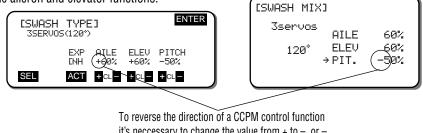
To reverse the direction of a CCPM control function it's neccessary to change the value from + to -, or to + as needed.
