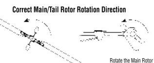
Rotate the Main Rotor counterclockwise (backward) and note the rotation of the Tail Rotor.
