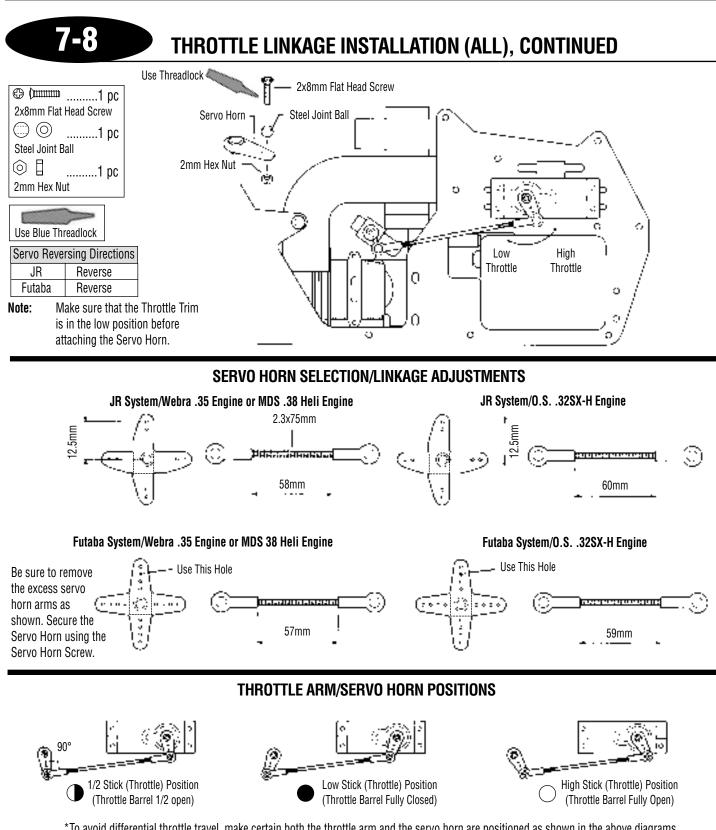
\*To avoid differential throttle travel, make certain both the throttle arm and the servo horn are positioned as shown in the above diagrams.
