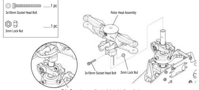
**Note:** Be sure to engage the rotor hub pin into the washout base groove before securing the rotor head in place
