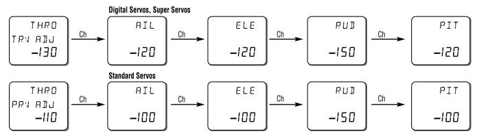
**Note:** The travel values shown for the rudder function are for use with Piezo gyros, like the JR NEJ-900, NEJ-400, NEJ-450, or NEJ-3000 type gyros. If a conventional mechanical type gyro is used (JR 120, 130, etc.), then the travel values of the rudder will need to be reduced to approximately 100%.
