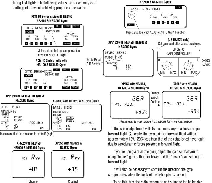
To do this, turn the radio system on and suspend the helicopter by the main rotor head. Next, move the rudder stick to the right and watch the direction that the tail rotor servo arm travels. Now while watching the tail rotor servo arm, rotate the body of the helicopter counterclockwise. The servo arm should move in the same direction as when the rudder stick was moved to the left. If the arm moves in the opposite direction, reverse the gyro and re-test.
